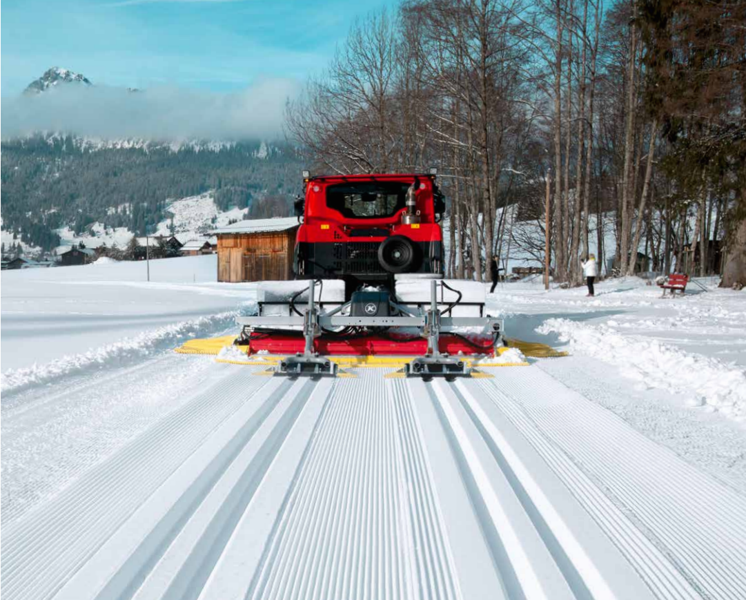
Mechanically adjustable 2-way track setter 2-way track setter with hydraulic adjustment on one side
