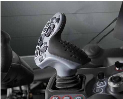
Joystick with ergonomic and proportional control for intuitive working.
