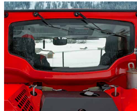
Larger and heated rear window for optimum visibility to the rear as well.
