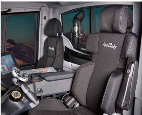
New ergonomic seat with improved lateral support, a wealth of adjustment options and seat heating.
