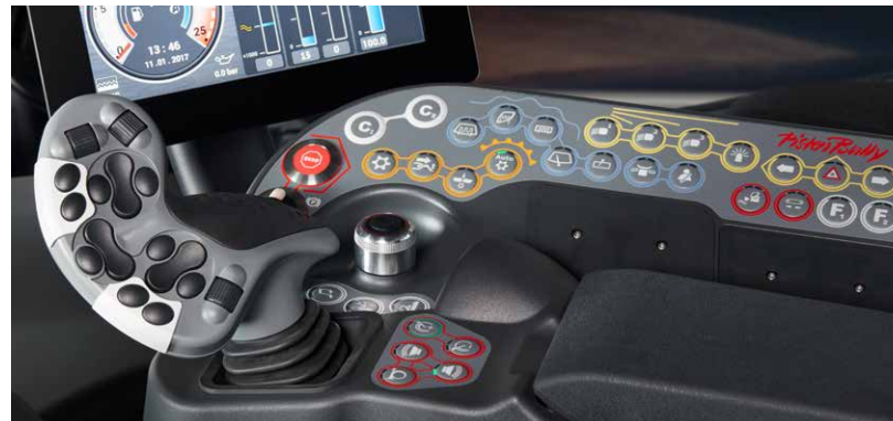
Armrest with convenient and individually programmable customer buttons.
