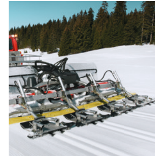
4-way track setter Professional track setter for preparation of 4 cross-country tracks at a time, such as are required for mass-start competitions.
