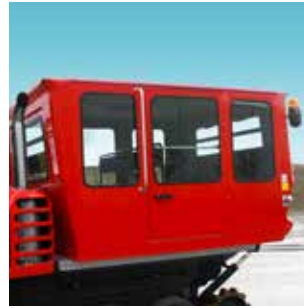
Cab 15 to 20 person / 1,600 kg Cab for moving up to 20 people with 2 foldaway benches and 2 fixed benches.
