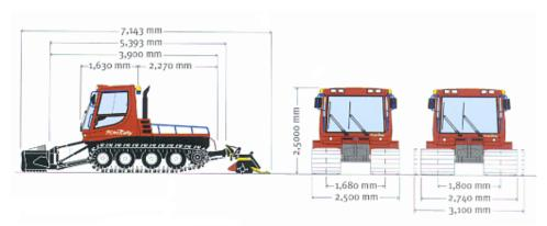
The PB 100 is available to two widths: 1,680 mm and 1,800 mm.
